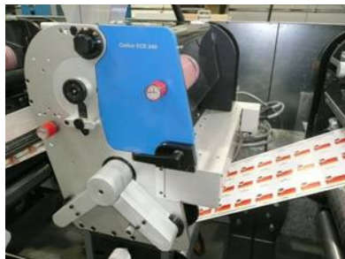
Figure 8: Narrow web flexo press using UV-LED
