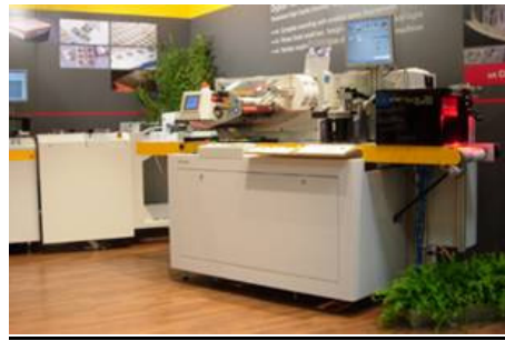
Figure 7: Example of Single Pass Printer using UV-LED
